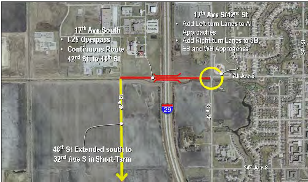
Figure 6-15: 17th Avenue Grade Separation Concept from 2035 LRTP
