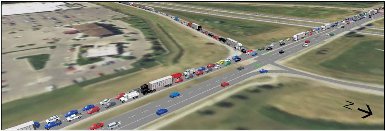
Figure 3-16: Queue Spillback during 2025 P.M. Peak at 32nd Avenue South/US81B
