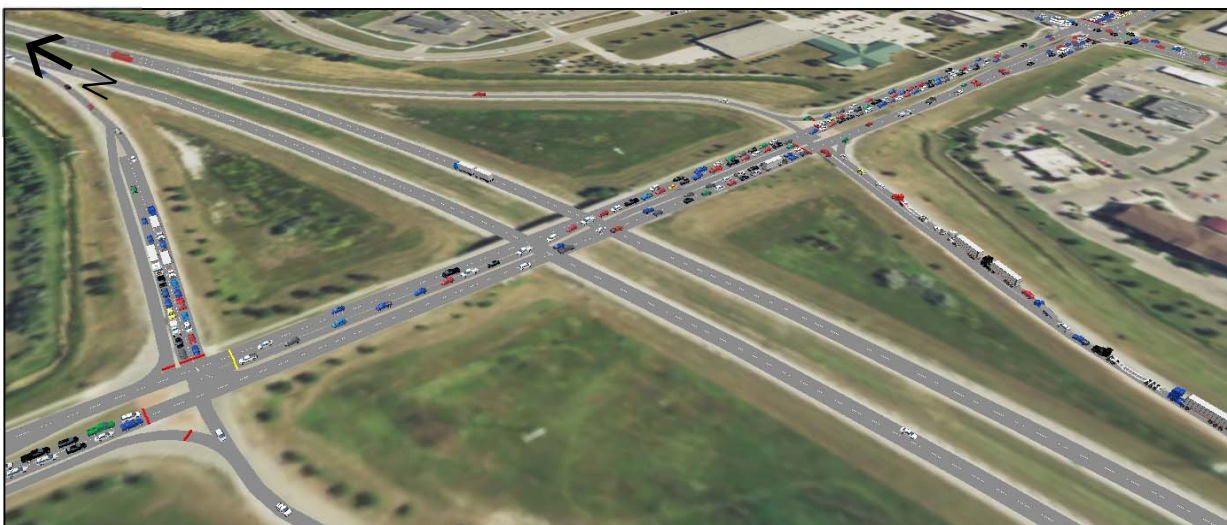
Figure 3-21: Queues Extend through Ramp Intersections at 32nd Avenue South/US 81B
