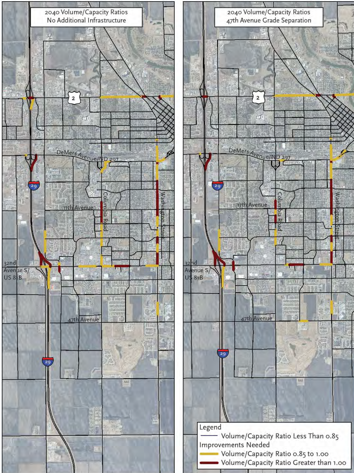
Figure 6-20: Volume/Capacity Ratios for Existing and Committed Network and 47th Avenue Grade Separation
