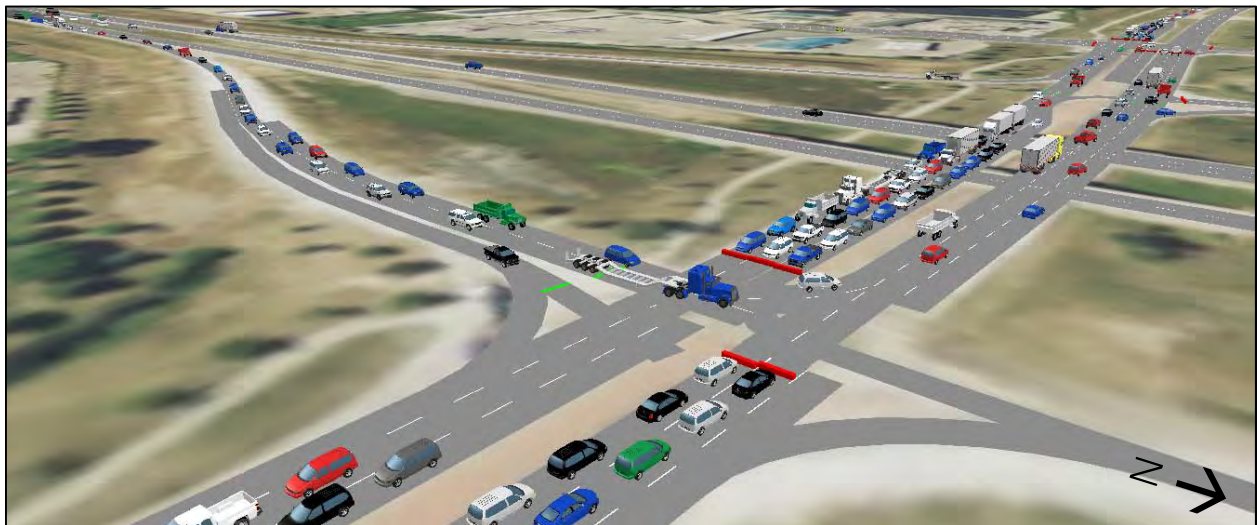
Figure 3-19: Queues Extend onto I-29 at the Gateway Drive/US 2 Interchange
