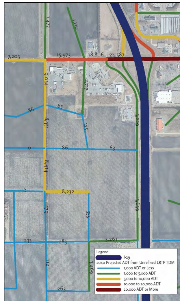
Figure 3-7: Projected 2040 ADTs from Unrefined L RTP TDM
