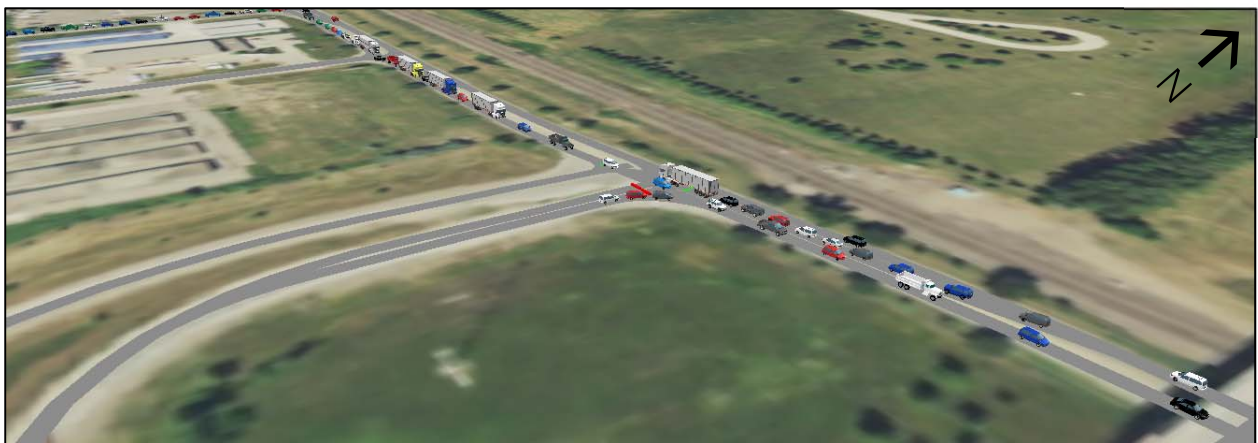
Figure 3-15: Eastbound Queues at the DeMers Avenue/ND 297 West Ramp Intersection during 2025 P.M. Peak
